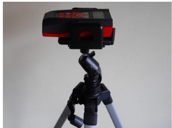
Fig. 2. Measuring device with the laser telemeter.
